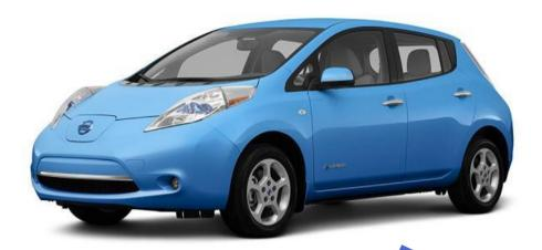
32.83kg copper used in a Nissan Leaf battery pack.
