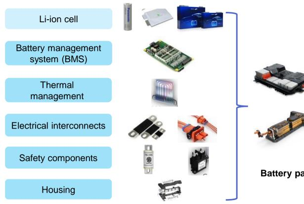
Note: Battery pack, together with power conditioning systems (PCS) including inverters, battery chargers, energy management systems, consist of a **battery** system.
